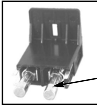
FUSES LOCATED IN VOLTAGE SELECTOR MODULE
