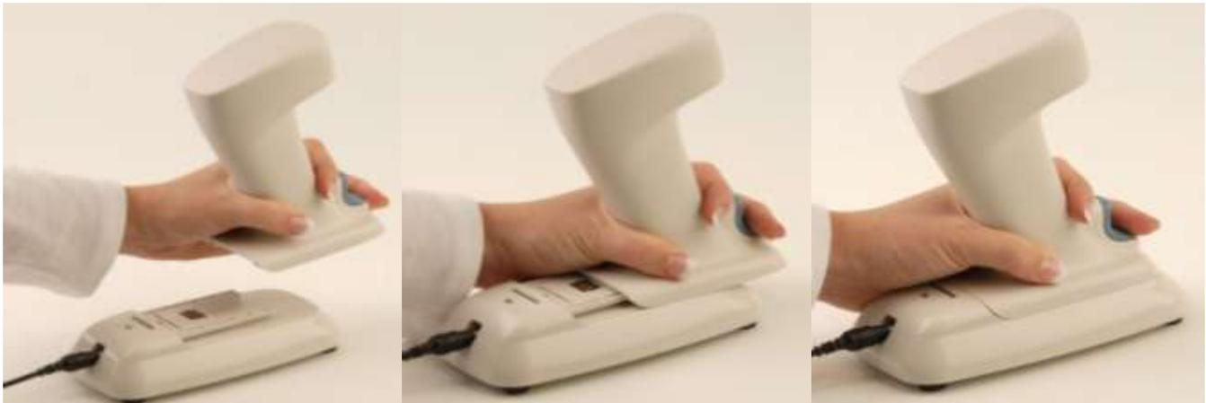
**2** Invert one of the handsets and carefully slide it onto the charging cradle (do not force the handset onto the charging cradle or damage may result). Expect charge time to be less than 3 hours. The handset, charging cradle, and AC power supply may become warm to the touch while charging. The handset may be left on the charging cradle overnight without damaging the batteries.
