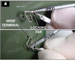
reinstalled. Use the small screw-driver to pry or push the tabs outward, as shown in Fig. 4.
