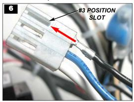
Reinstall the 3-Wire Connector onto the 'J3' 3-pin receptacle located on the PC Board, as shown in
