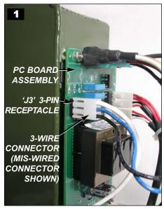
3-pin receptacle on the Board (Fig. 1).
