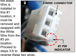
Insert a small, thin screwdriver into the #1-pin slot located on the side of the 3-Wire Connector and
