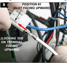
Repeat the procedure above in Step 5 for the Black Wire (Fig. 6). Assure that the black, white, and blue wires are secured firmly into the 3-Wire Connector.
