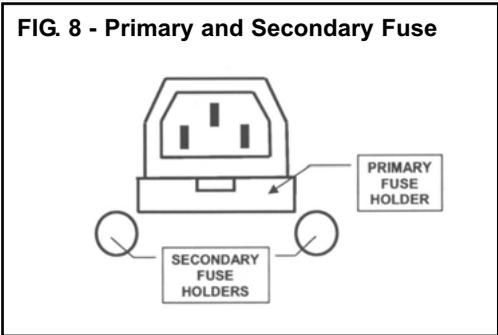
**FIG. 8 - Primary and Secondary Fuse**
